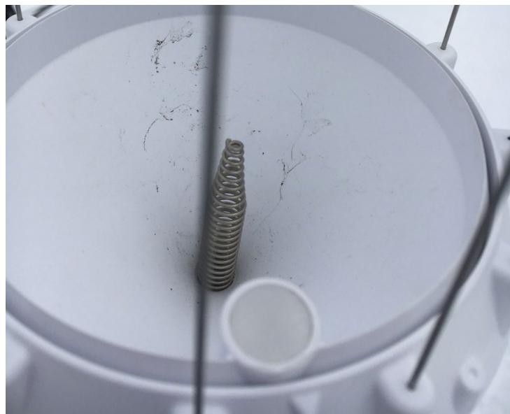
Figure 3: Incorrect installation: sensor is slightly offset from the triangle.
