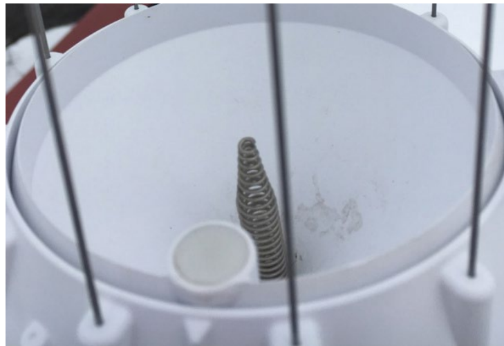
Figure 2: Correct installation: sensor is centered at the triangle.
