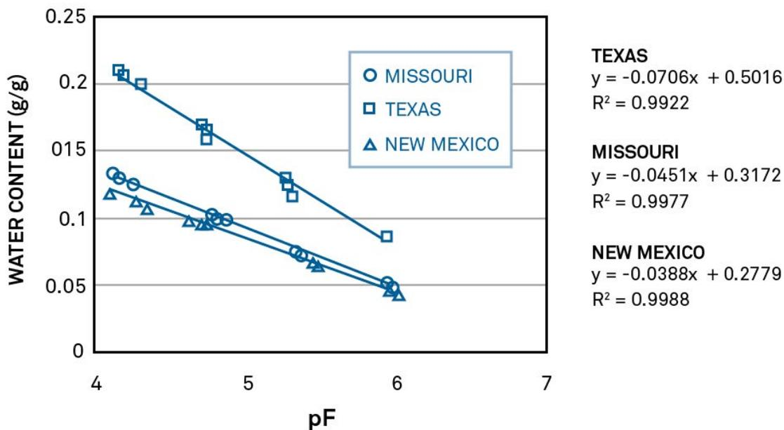
Figure 1. Table 1 gives the McKen classification scheme. The second column shows the slope range for each group. For the three soils in the figure, the Missouri and New Mexico samples fall in class V, which are non-expansive. The Texas sample is class IV, which is a low expansion.
