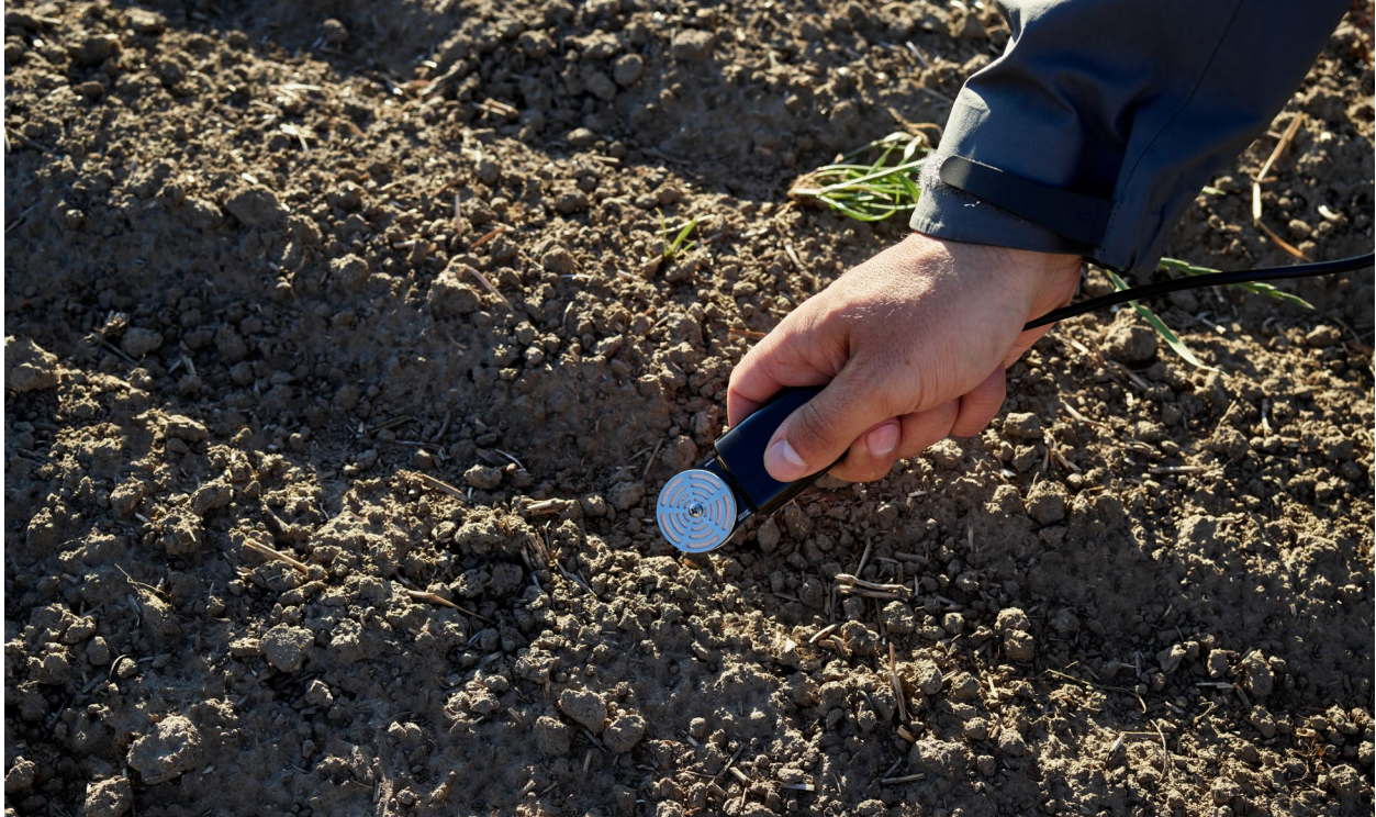
METER TEROS 21 water potential sensor
