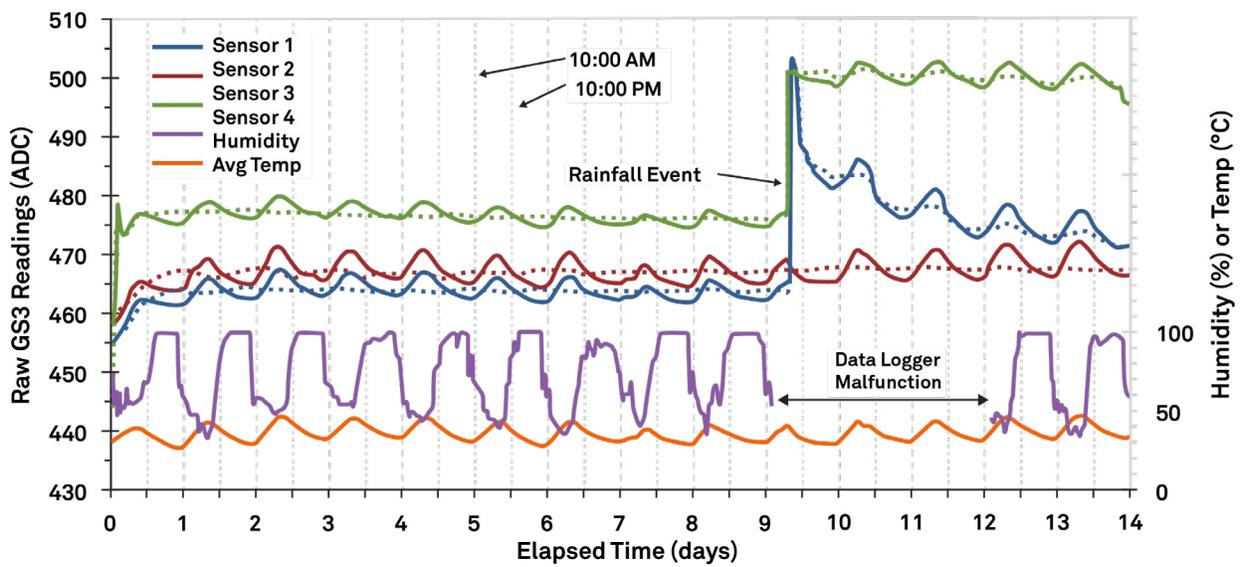
Figure 3b. Unprocessed GS3 moisture data during 14-day curing period alongside temperature and humidity from Hwy. 45 Alt (Cox et al., 2015)
