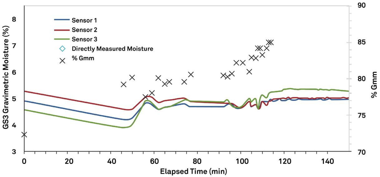
Figure 4a. Processed GS3 gravimetric moisture data during compaction alongside corrected NG densities from Hwy. 45 Alt (Cox et al., 2015)
