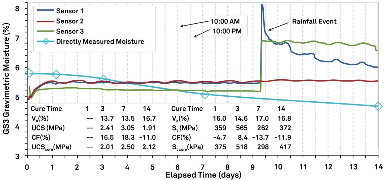
Figure 4b. Processed GS3 gravimetric moisture data during 14-day curing period alongside directly measured core properties from Hwy. 45 Alt (Cox et al., 2015)
