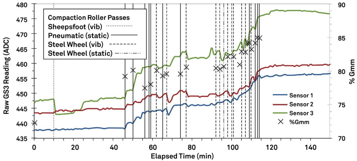
Figure 3a. Unprocessed GS3 moisture data during compaction alongside roller passes and corrected NG densities from Hwy. 45 Alt (Cox et al., 2015)
