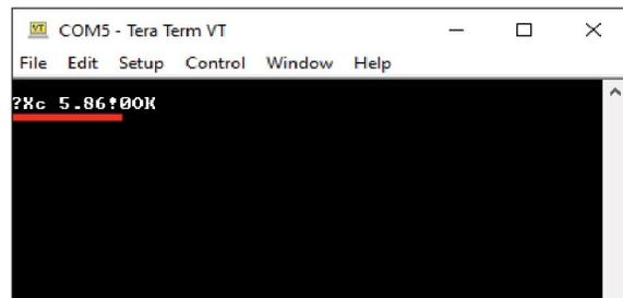
Figure 31. Enter CAL Factor value for replacement funnel
