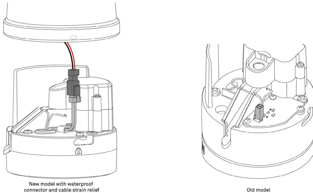
Figure 1. Rain funnel and pyranometer connector
