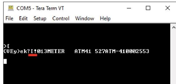
Figure 30. Enter direct communication mode
