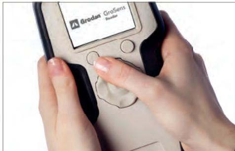
Push the top left button to switch on the reader
