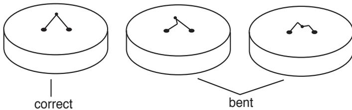
*Figure 11: Proper thermocouple position*
