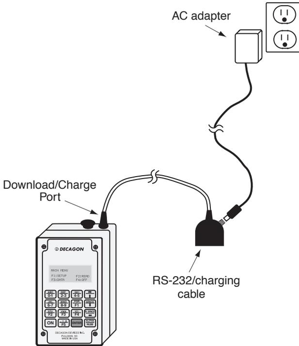
*Figure 4: Recharge setup*
