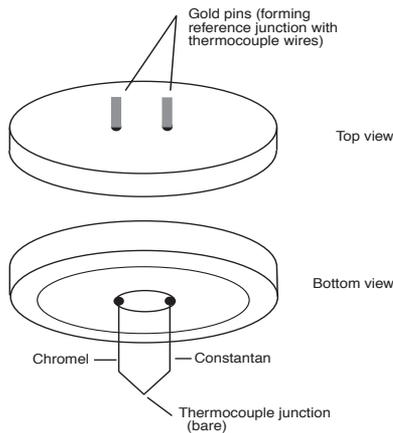
*Figure 7: Peltier thermocouple*
