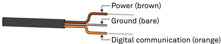
Figure 2 Pigtail wiring
