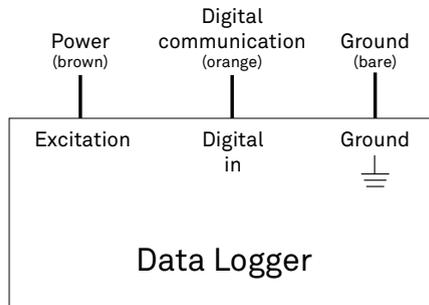
Figure 3 Wiring diagram
