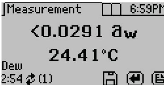
Figure 1 Low water activity reading
