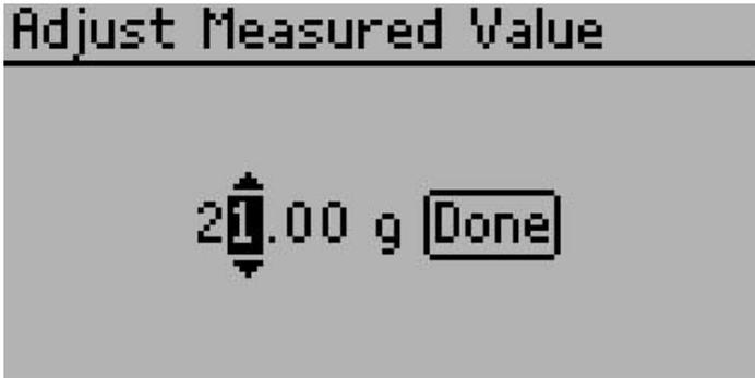
Operators may run the calibration sequence as frequently as necessary to ensure and verify they are taking accurate readings. Once the calibration is complete, the new value stores in the Infiltrrometer Firmware and does not erase until you set a new calibration setting.
