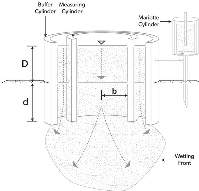
Figure 15: Cross Section of a Double-Ring Infiltrometer
