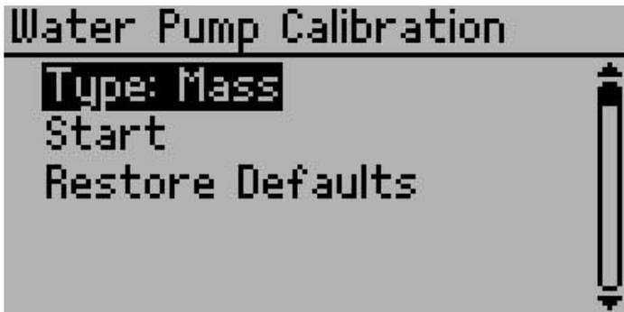
To calibrate pump, first Select Menu > Configuration > Water Pump Calibration. Select Type, either mass or volume, highlight Start, and press Enter. You should receive a message to connect a water source and attach the outgoing water tube. Connect a source of water and press Enter.
