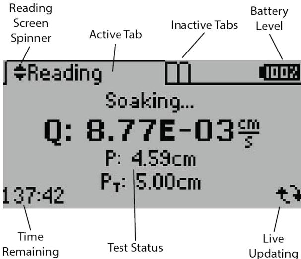
Figure 9: Reading Screen Breakdown
