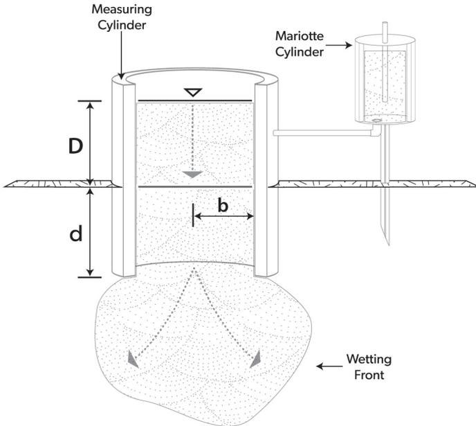
Figure 14: Cross Section of a Single-Ring Infiltrometer
