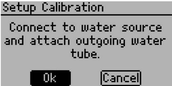
Both methods require that you first purge the water line of any air before running the calibration. The screen reminds you to purge the tube, highlight purge, press Enter. Keep running water through until water runs clear with no bubbles. For the mass method, tare the scale with your water reservoir after you finish purging the line of all air.
