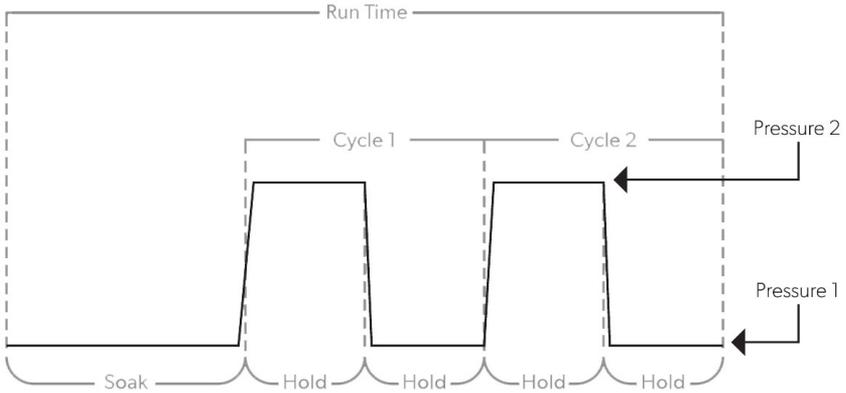
Figure 10: Run Time Diagram
