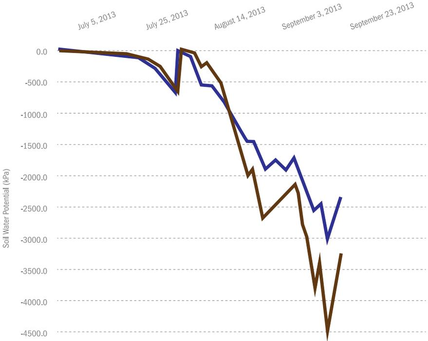
Figure 4: Time series MPS water potential data collected at 20 cm under a dry oak forest in Switzerland. Note the range extends well beyond permanent wilting point.<sup>3</sup>
