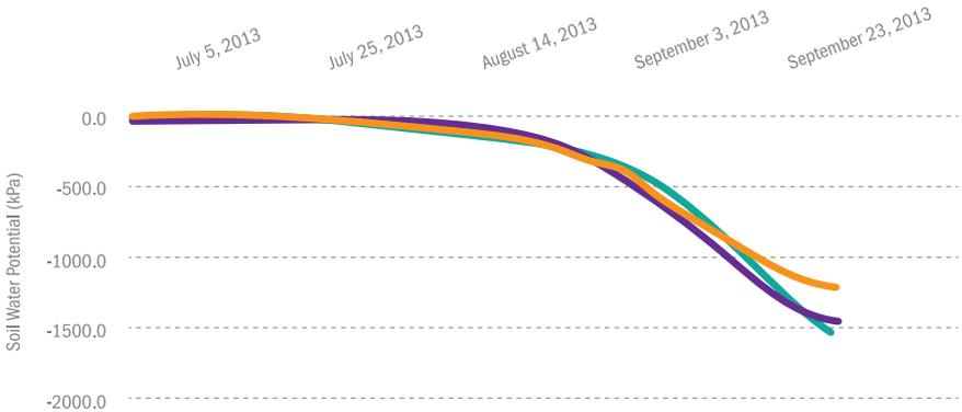
Figure 3: Time series MPS water potential data collected at 80 cm depth under a Beech forest in Switzerland. Note the excellent sensor agreement down to permanent wilting point ( $-1,500$  KPa).<sup>3</sup>
