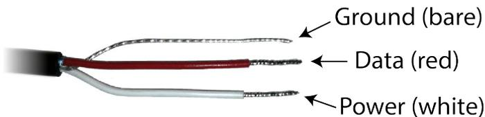
Figure 6: Pigtail End Wiring
