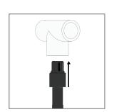
Tank or Water Body Installation. Suspend the sensor in the tank or water body away from the sides of the tank or water body as much as possible.
