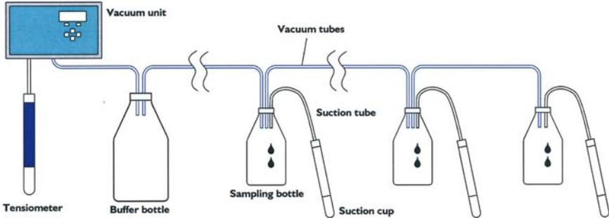
*Fig: Sampling bottles connected in row using 3<sup>rd</sup> nozzle on the cap*
