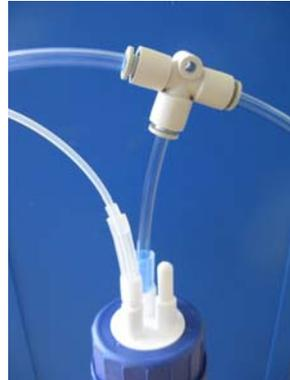
The purpose of the overflow protection is to prevent damages to the vacuum unit and to avoid that solution from one bottle contaminates other bottles in case of unexpected incidents. It is not intended as an automatic stop switch, mainly because the membrane has to completely dry off before it again is permeable to vacuum.
