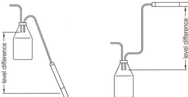
Accordingly, if the sampling bottle is lower than the suction cup, for example in a manhole (right figure), the effective vacuum on the sampler is higher than inside the bottle - if the tube is completely filled with water. In a normal situation there will be vapor and bubbles inside the tube. Therefore, you do not reduce the vacuum so solution is extracted even with bubbles inside the tube.
