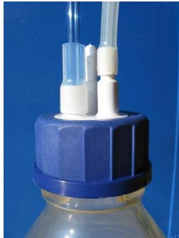
The third nozzle is not open but optionally can be used for connecting another suction tube or to conduct the vacuum to another sampling bottle. To do so, cut off the tip of the nozzle. Cut off the upmost section for a thin suction tube or the lower section for a thicker vacuum tube.
