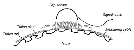
Scheme of the installed D6
