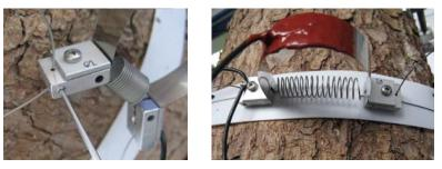
Lead the measuring steel cable around the trunk and cut it off with the required length. The length should be 5 cm longer than the circumference to allow a readjustment of the cable when the end of the measuring range is reached.
