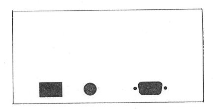
The rear panel shown above has the on/off power switch at the left, the 12 volt do power input jack in the middle and the RS232 I/O port on the right.
