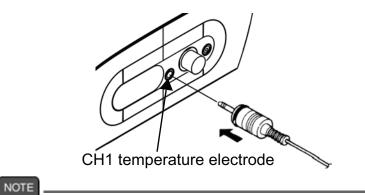
If the temperature connector is unconnected or the connection is wrong, the MTC set temperature is displayed as the sample temperature.
