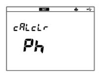
Press the ENTER key to enter the calibration data deleting (Yes/No) screen.
