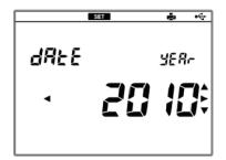
Press the ◀ or ▶ key to select a digit and press the ▲ or ▼ key to change the value for month and day setting, and then press the ENTER key.
