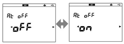
6. Press the ◀ or ▶ key to select a digit and press the ▲ or ▼ key to change the value, and then press the ENTER key to return to the auto power off change screen.
