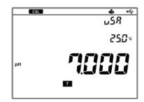
The **7** mark, which means that the pH7 calibration is completed, is displayed on the screen.
