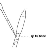
**5.** Wash the tip of the electrode well with pure water (deionized) and wipe it with filter or tissue paper.
