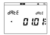
6. Press the ◀ or ▶ key to select a digit and press the ▲ or ▼ key to change the value for hour and minute setting, and press the ENTER key to return to the date setting screen.
