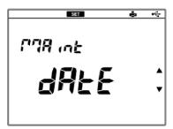
Press the ENTER key to enter the year setting screen. Press the ◄ or ► key to select a digit and press the ▲ or ▼ key to change the value, and then press the ENTER key.
