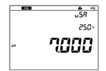
**5.** Check the stable indication value, and press the CAL key.
