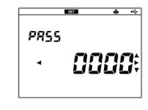
If this setting is ON, password entry is required when you power ON the instrument. Enter the password and press the ENTER key.
