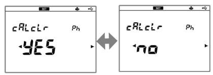
Press the ◀ or ► key to select Yes, and press ENTER key to delete the calibration data.
