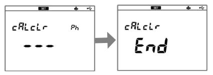
**7.** Press the ENTER key to return to the calibration data clear screen.
