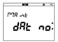
**4.** Press the ENTER key to display the number of the memory data currently saved in the instrument.
