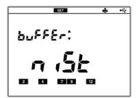
**2.** Press the ENTER key to enter the pH standard solution change screen
