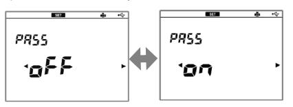
6. If you select ON, press the ◀ or ▶ key to select a digit and press the ▲ or ▼ key to change the value, and then press the ENTER key and press the ENTER key to return to the password change screen.
