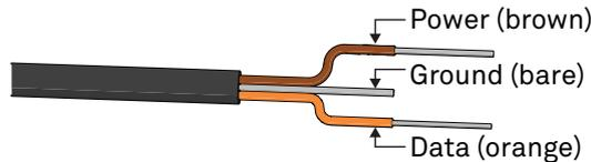
Figure 3 Pigtail wiring
