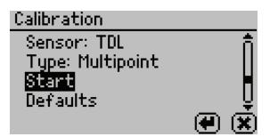
Figure 52 TDL sensor calibration screen
