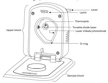
Figure 62 AQUALAB TDL sample chamber diagram
