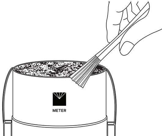
Figure 49 Fix and clean the soil sampling ring
