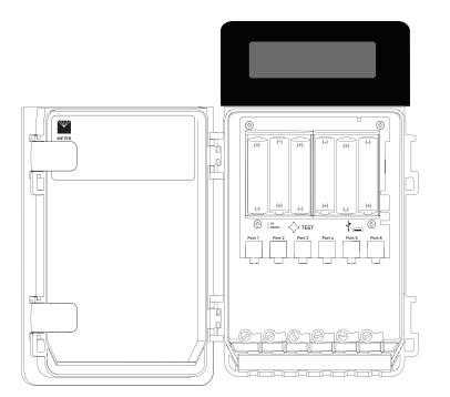
Figure 15 ZL6 data logger interior
