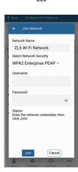
Figure 20 Configuration of an enterprise network
