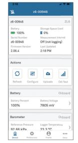
Figure 9 ZL6 information and current sensor readings
