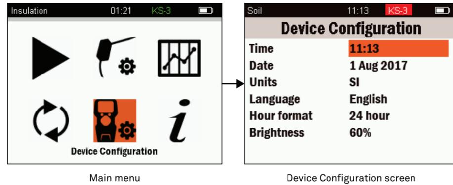
Figure 10 Device Configuration screen
