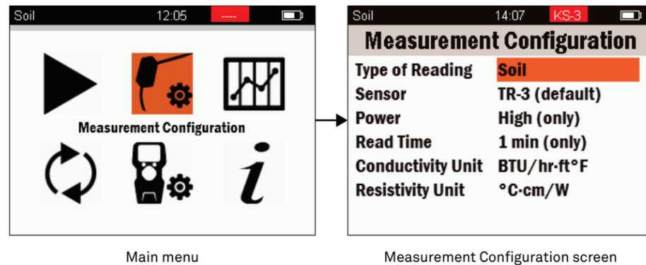
Figure 19 Measurement Configuration screen
