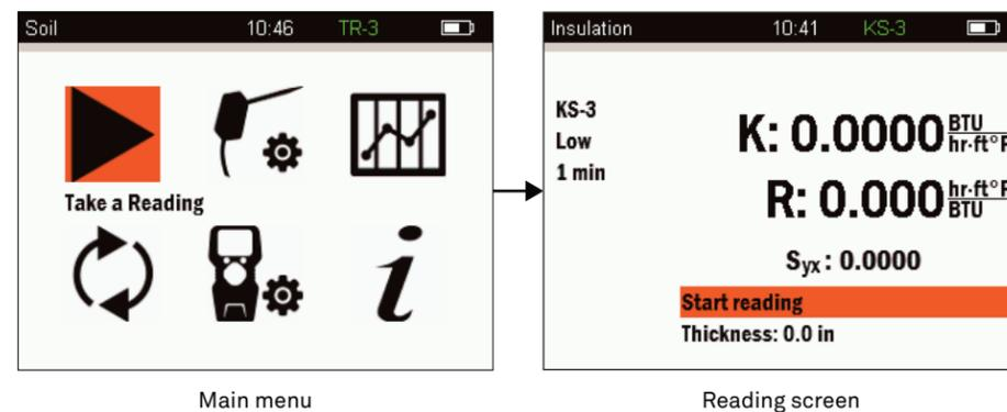
Figure 4 Navigating to the Take a Reading screen
