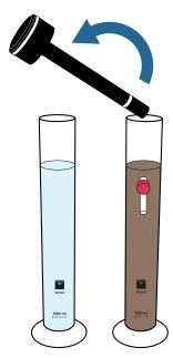
Figure 15 Replace PARIO in distilled water after test
