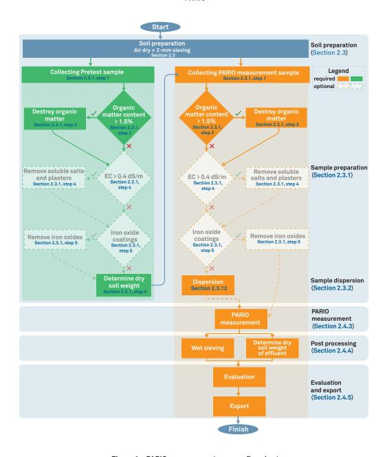
Figure 1 PARIO measurement process flowchart
