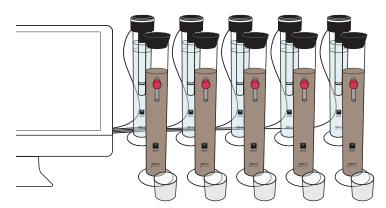
Figure 2 Schematic of workbench with standby cylinders, sedimentation cylinders, and beakers for PARIO Plus analysis
