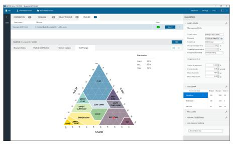
Figure A.4 Example silt loam soil triangle results
