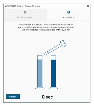
Figure 11 Completed PARIO Control countdown with instructions to insert PARIO into sedimentation cylinder
