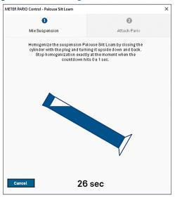
Figure 9 PARIO Control homogenization countdown with mixing instructions
