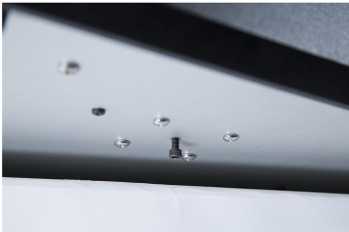
Figure 6: Loosened Shipping Screw
