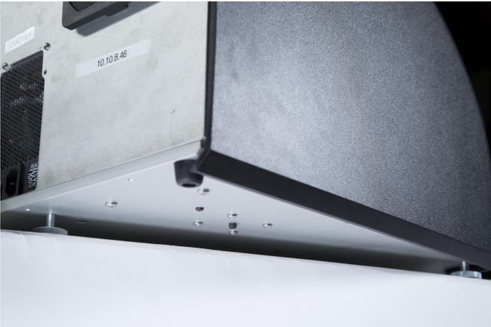
Figure 5: Locate Shipping Screw
