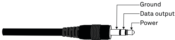
Figure 2 3.5-mm stereo plug connector wiring
