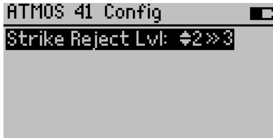
Figure 24 Adjusting the ATMOS 41 strike reject level
