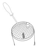
To remove the particulate screen, use a small blunt object such as a screwdriver to gently pry up from the edge of the screen.
