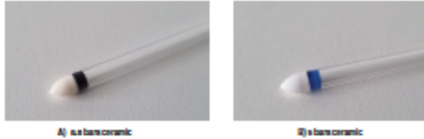
Figure 1 Tensiometer shafts (A) 0.5-bar ceramic (B) 5-bar ceramic
