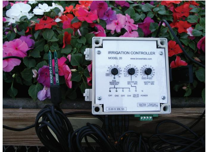
*Figure 4. We developed an automated irrigation controller in cooperation with Brower Electronics Laboratories. This controller uses 1 to 4 ECH20 probes to control irrigation based on grower-determined set points.*
