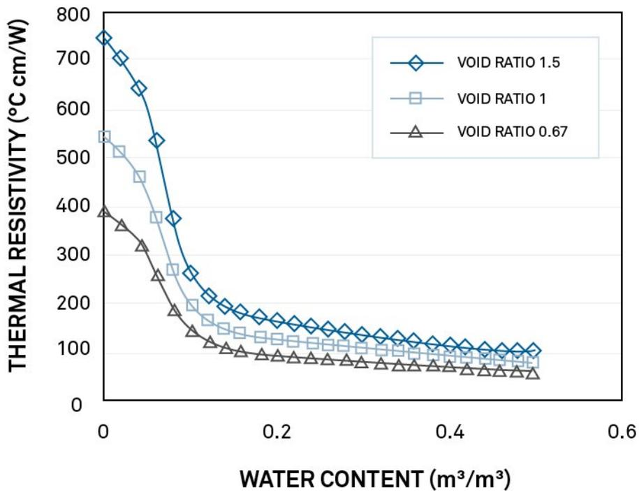
Figure 2. Effect of density and water content on thermal resistivity of a loam soil. The void ratio 1 curve is the same as in Figure 1. The bulk densities are 1.06 Mg/m<sup>3</sup> for void ratio of 1.5, 1.33 Mg/m<sup>3</sup> for void ratio 1, and 1.59 Mg/m<sup>3</sup> for void ratio of 0.67.
