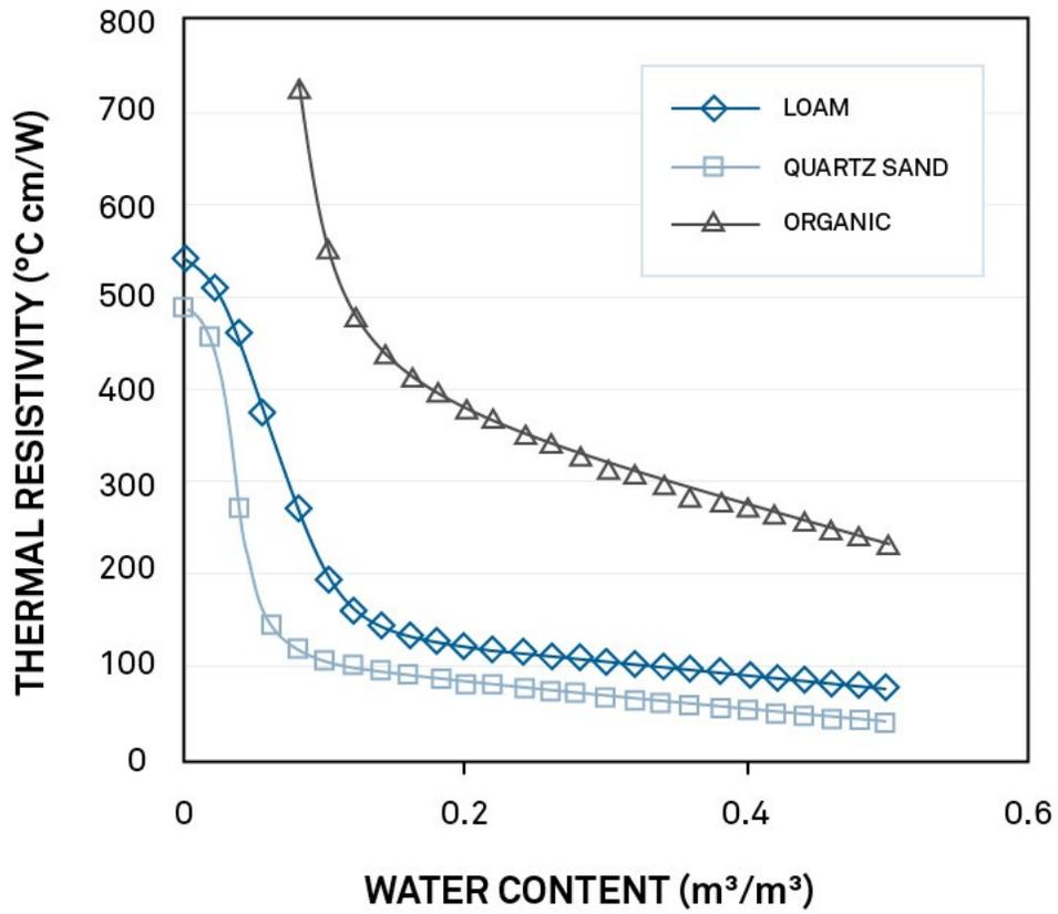
Figure 1. The thermal resistivity of 3 soil materials as a function of water content. The solid fraction in each was 0.5.
