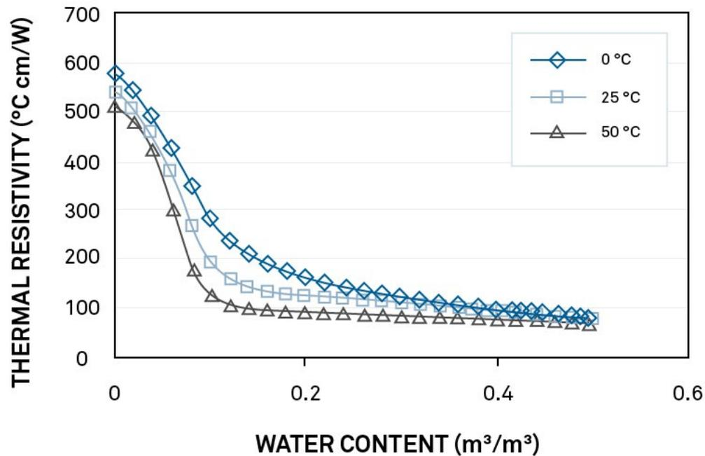
Figure 3. Effect of temperature and water content on thermal resistivity of a loam soil. The 25 °C curve is the same as in Figure 1
