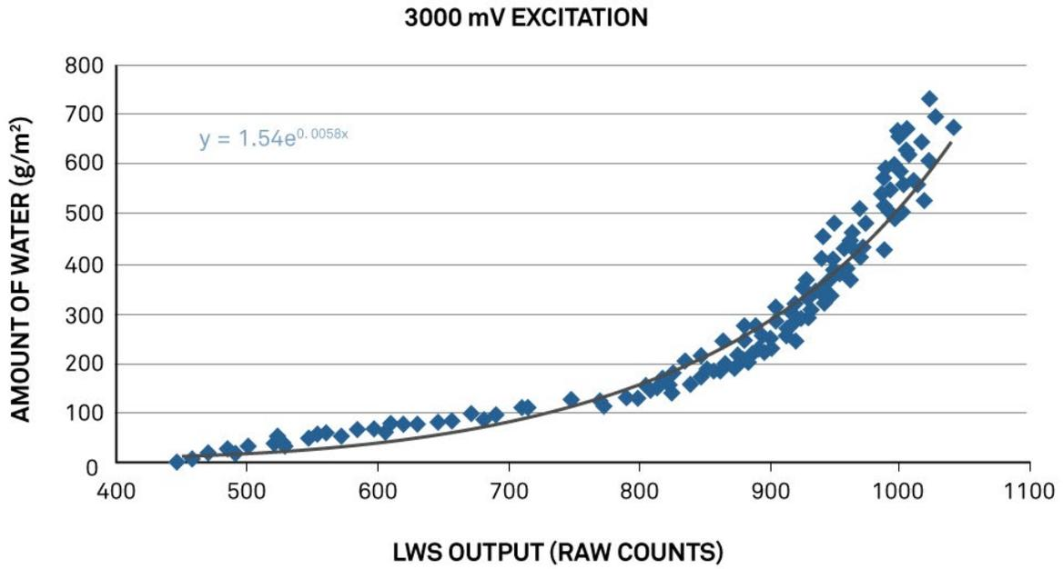
Figure 1. Amount of water on PHYTOS 31 surface as a function of PHYTOS 31 raw counts measured with METER EM50 series data logger
