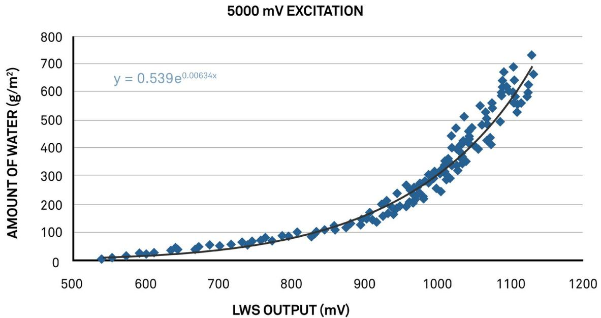
Figure 3. Amount of water on PHYTOS 31 surface as a function of PHYTOS 31 mV output when excited at 5000 mV
