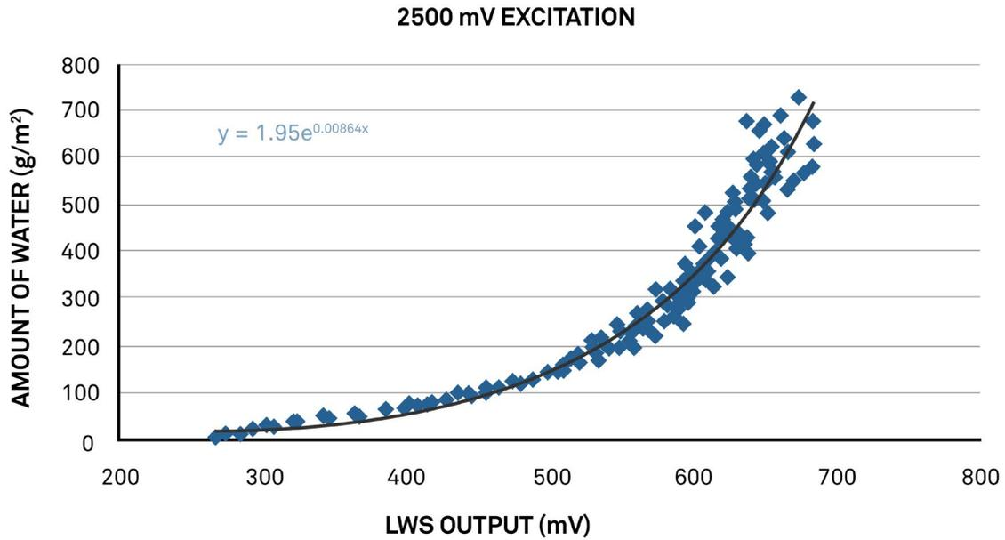
Figure 2. Amount of water on PHYTOS 31 surface as a function of PHYTOS 31 mV output when excited at 2500 mV. This relationship can be used with Campbell Scientific or other third-party data acquisition systems that excite the PHYTOS 31 at 2500 mV.
