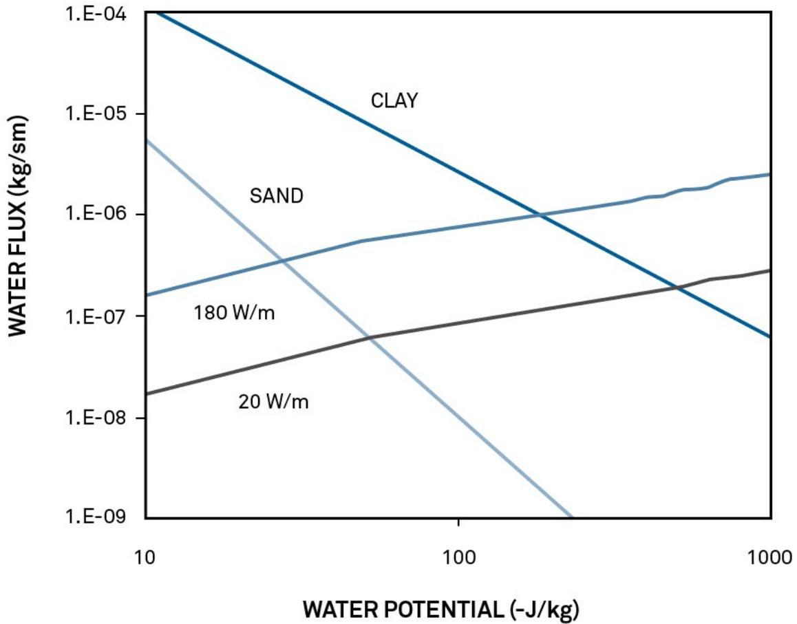
Figure 1. Graph of Equation 4 and Equation 10 for sand and clay liquid flow estimates and high and low heat dissipation rates
