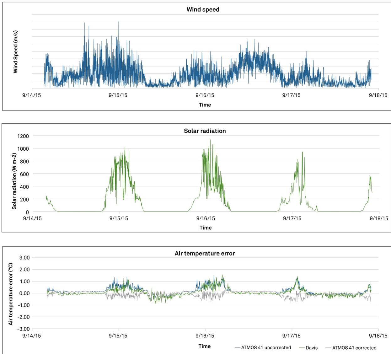
Figure 1. Environmental conditions and air temperature error ( $T_{\text{measured}} - T_{\text{TS-100}}$ ) for the two air temperature sensors under evaluation
