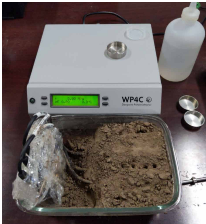
Figure 3. WP4C and soil container with TEROS-21 sensors and augered sample removed.
