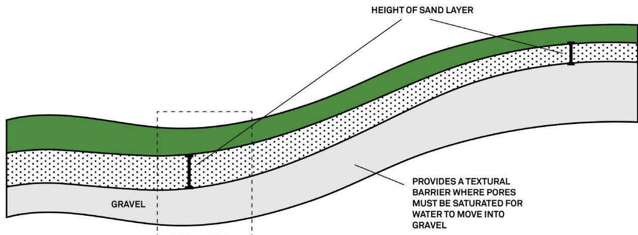
Figure 1. Diagram of sand and gravel layers beneath a putting green
