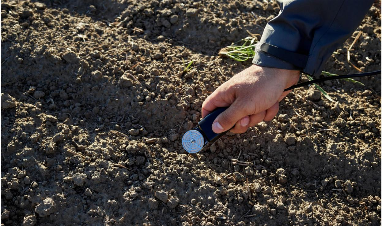
[TEROS 21](#) field water potential sensor measures [water availability](#) which is critical for [irrigation scheduling](#)
