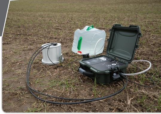
The new fully automated DualHead Infiltrometer measures ( $K_{fs}$ ), the ability of a porous medium to transmit water under saturated or nearly saturated conditions. The DualHead Infiltrometer uses the multiple head analysis approach to correct 3-dimensional flow without having to guess the Soil Sorptivity (S) and the Soil Macroscopic Capillary Length ( $\alpha$ ).
