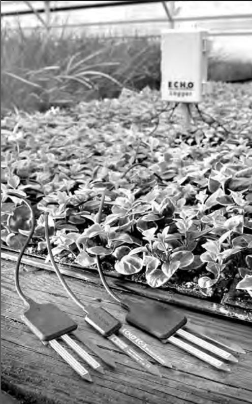
■ The new ECH<sub>2</sub>O-5 measures the volumetric water content of growth media and soil. Its compact, durable design make it an ideal soil moisture monitor for any setting, whether in the greenhouse or the field. The ECH<sub>2</sub>O-5 outputs a millivolt value from the probe, which is correlated with water content.
