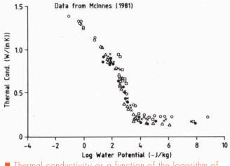
Thermal conductivity as a function of the logarithm of water potential for soils ranging from sand to clay.
