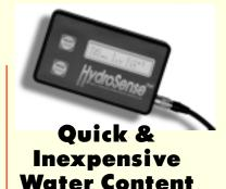
HydroSense measures volumetric water content: 0 to Saturation in 0.5 seconds. Measurement units: Percent volumetric water content. Resolution: 1.0%. Accuracy: ±3.0% volumetric water content with electrical conductivity <2 dS m<sup>-1</sup>. Range: 0% to saturation. Saturation is typically around 50% volumetric water. Stabilization: Instantaneous. Response time: <50 ms.
