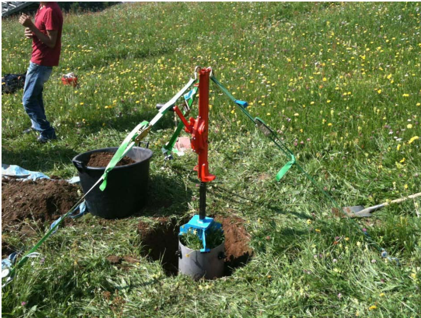
Soil column cutting with jack lift device
