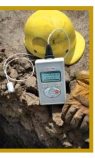
The KD2 Pro with the TR-1 needle can accurately measure the thermal conductivity/ resistivity of particles as large as coarse sand (1 mm diameter). Larger materials can cause problems for
