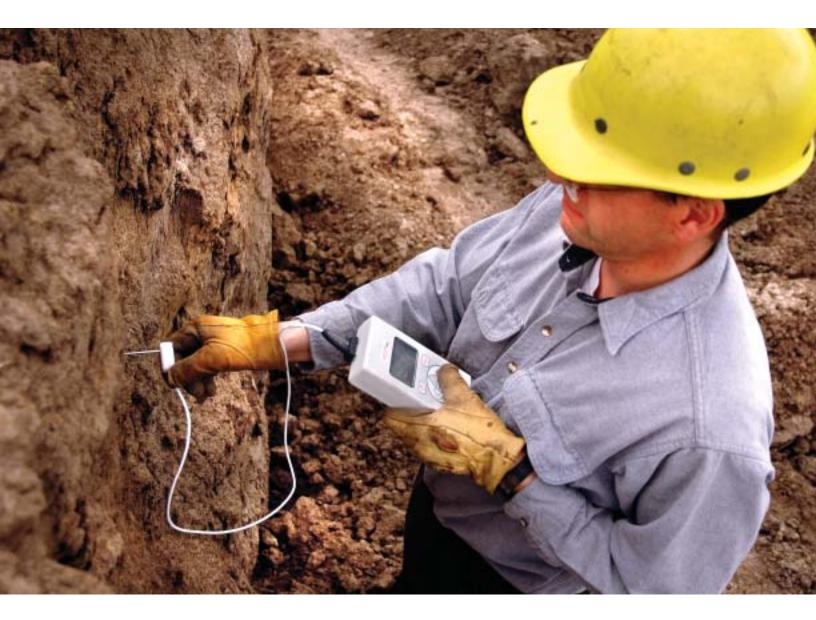
The KD2 Pro with the TR-1 needle can accurately measure the thermal conductivity/resistivity of particles as large as coarse sand (1 mm diameter).
