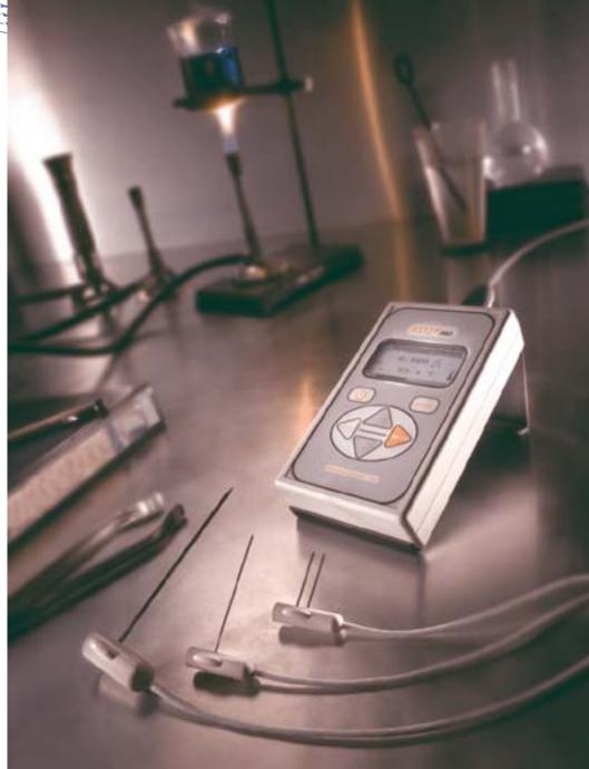
seems a little too good to be true. Does it possibly have some serious limitations? "Well," admits Bryan Wacker, head of Decagon's Research Instruments division, "you can't stick a needle into a rock." Because the KD2 Pro probe must be inserted into the sample, certain samples can't be read at all. And other samples are subject to "contact resistance errors," meaning that what the probe can't adequately touch and heat, it can't
