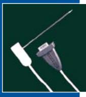
TR-1 (10 cm sensor) The TR-1 measures thermal conductivity and thermal resistivity and conforms to IEEE Standard 442-1981 and ASTM Standard D 5334-00
