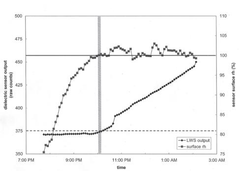
**Figure 3.** Sensor output and surface relative humidity of an out-of-the-box dielectric leaf wetness sensor over the onset of evening dew. The dashed horizontal line indicates the dry baseline output of the sensor, with anything greater than that threshold indicating surface wetness. The solid horizontal line indicates 100%  $rh_s$  when dew will just begin to form on the sensor surface. The gray zone indicates the time duration when the sensor indicates liquid water, but none is present.
