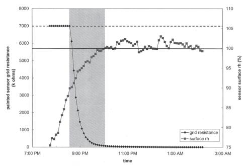
**Figure 2.** Grid resistance and surface relative humidity of a painted, baked resistance grid leaf wetness sensor over the onset of evening dew. The dashed horizontal line indicates the dry resistance of the sensor, with anything less than that threshold indicating surface wetness. The solid horizontal line indicates 100%  $rh_s$  when dew will just begin to form on the sensor surface. The gray zone indicates the time duration when the sensor indicates liquid water, but none is present.
