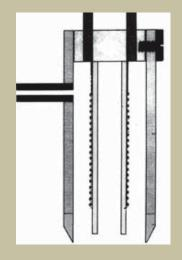
Ellis Wallihan's porometer design with the Dunmore electronic humidity sensor (circa 1960.)
