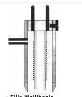
◆ Ellis Wallihan's porometer design with the Dunmore electronic humidity sensor (circa 1960.)
