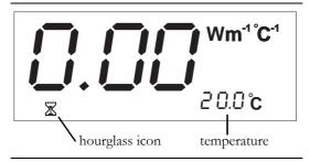
**Note!** Make sure to watch the temperature during the equilibration stage to make sure it doesn't drastically fluctuate or rapidly change. If the temperature is still rapidly changing, pull the probe out of the sample and wait until the sample temperature is stable before measuring again.
