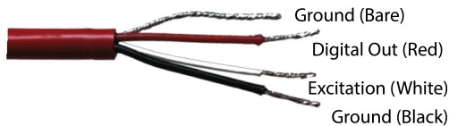
Figure 8: Pigtail End Wiring
