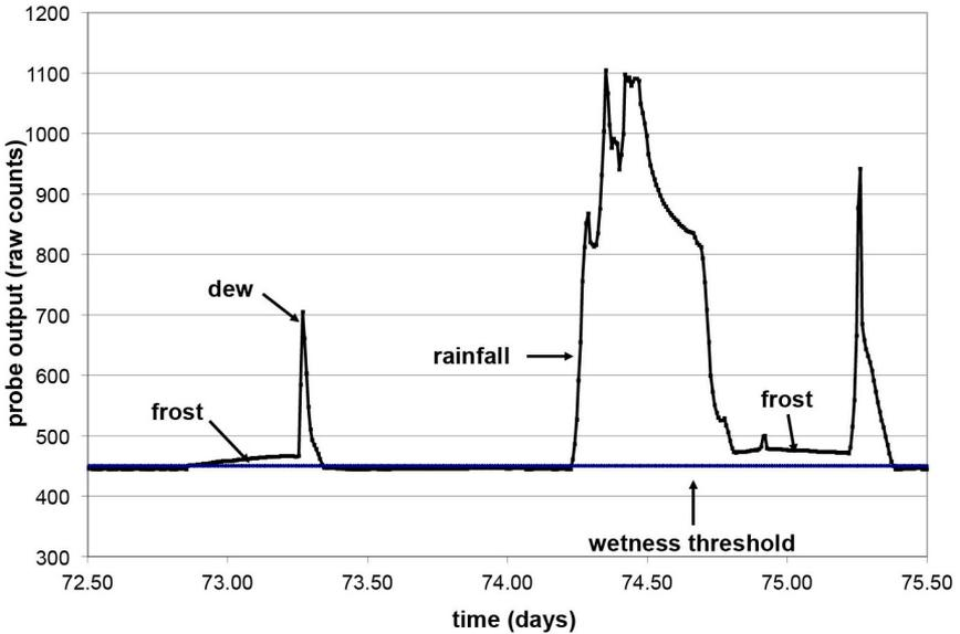
Figure 4: Sample raw output from the LWS
