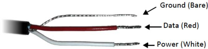
Figure 3: Sensor wiring diagram
