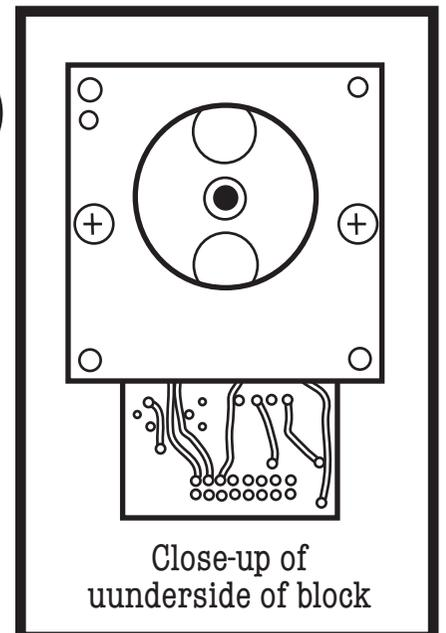
If the sensor is quite sticky, it is usually necessary to clean the bottom of the sample temperature sensor with alcohol.
