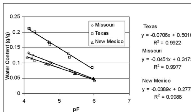
Table 1 on the next page gives the McKeen classification scheme. The second column shows the slope range for each group. For the three soils in the figure, the Missouri and New Mexico samples fall in class V, which are non-expansive. The Texas sample is class IV, which is a low expansion.
