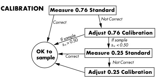
This flowchart is a graphical representation of the directions given below for verification of calibration.
